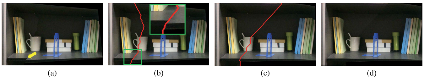
FIGURE 13. An extremely challenging scene for image stitching, in which two challenges occur at the same time. Images to be stitched lack rich texture and have large parallax either. (a) initial stitching result produced by seamline searching. It suffers obvious misalignment (as yellow arrow indicates). (b) result produced by SEAGULL [43]. Misalignment artifacts are not effectively eliminated. (c) result produced by proposed method. (d) final stitching result after image blending.
