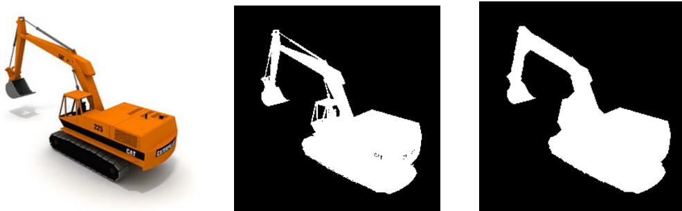
FIGURE 2. Binary image optimization. The first image is the original image, the second image is the first processed binary image and the last image is the second processed binary images.
