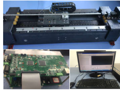
FIGURE 5. PMLSM drive platform.
