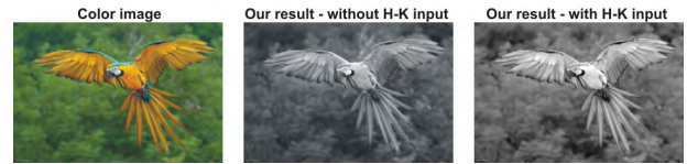
FIGURE 4. Importance of the Helmholtz-Kohlrausch ( H - K ) input to improve the contrast of our decolorized result.
