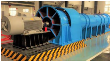
FIGURE 11. Fan aerodynamic performance of the test platform.
