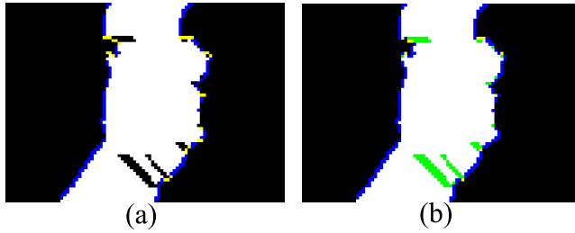
FIGURE 15. Restoration of discontinued parts of an edge through: (a) Connection of discontinued parts of the edge; (b) Restored crack region after the hole filling operation (■ detected edge, ■ connected edge, ■ restored edge).
