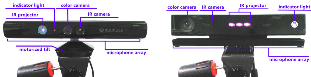
FIGURE 1. Two different structures of Microsoft Kinect: (a) Kinect v1 and (b) Kinect v2.
