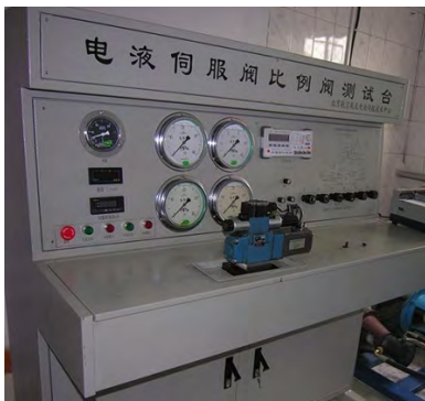
FIGURE 14. Experimental test bench of electro-hydraulic servo valve.
