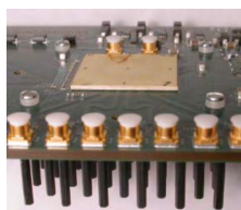
FIGURE 6. Package mounted on evaluation board with heat sink (taken from [48]).
