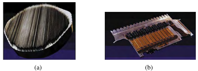
FIGURE 4. An airborne phased array radar antenna (taken from [46]), (a) array aperture, (b) a row of microwave modules on a slat.
