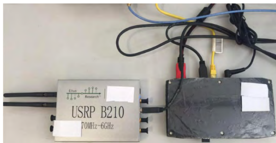
FIGURE 25. The software-defined device composed by USRP-B210 and INTEL NUC.
