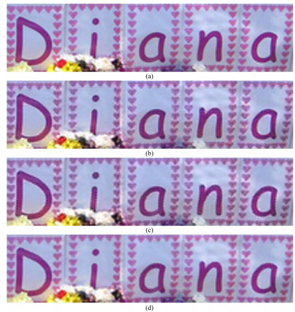
FIGURE 20. Comparison of (a) original image and result of the (b) AHD, (c) HOI, and (h) Proposed methods (LC #5).
