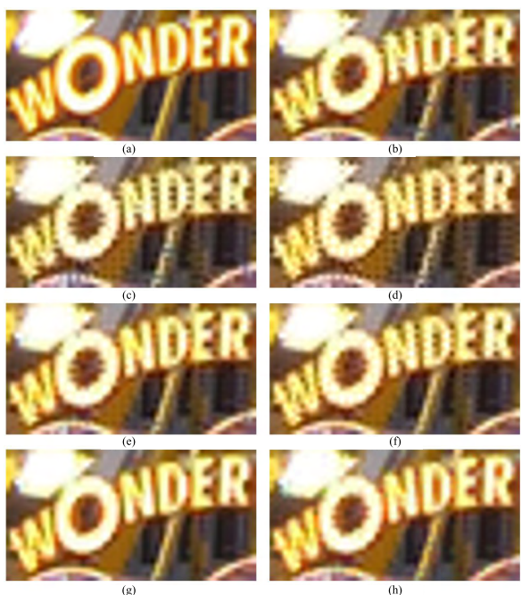
FIGURE 14. Comparison of (a) original image and result of the (b) VCD, (c) EDUSC, (d) ESF, (e) EDAEP, (f) CDDFW, (g) VDI, and (h) Proposed methods (LC #3).
