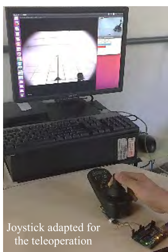
FIGURE 16. Experiment with the teleoperation by the joystick control interface.
