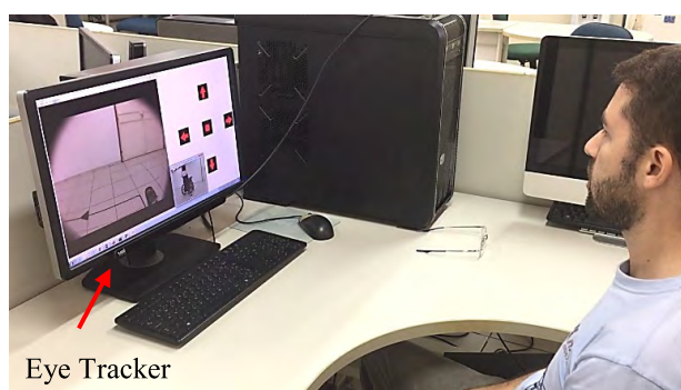
FIGURE 17. Experiment with teleoperation by the eye tracker control interface.
