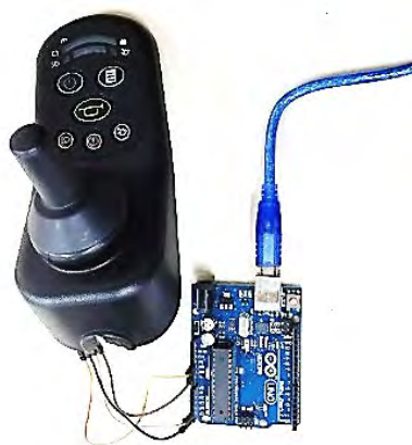
FIGURE 4. Original EPW joystick adapted to teleoperate by distance.
