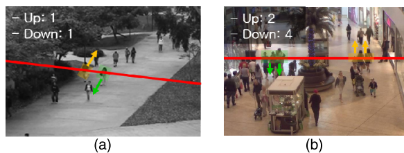
FIGURE 2. Example of people counting approach based on the line of interest (red solid line). (a) Frame from the Grand Central dataset [6]. (b) Frame from the University of California, San Diego (UCSD) dataset [2].
