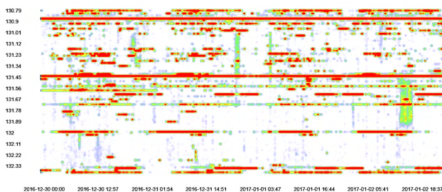
FIGURE 14. Signal heat map. The horizontal coordinate is time and the vertical coordinate is frequency.
