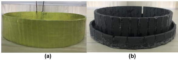
FIGURE 13. The magnetic coupling part model of wireless power transfer system for monitoring devices. (a) The coil. (b) The optimized magnetic core structure.
