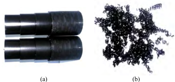
FIGURE 2. (a) Machined specimen and (b) chips during the machining.
