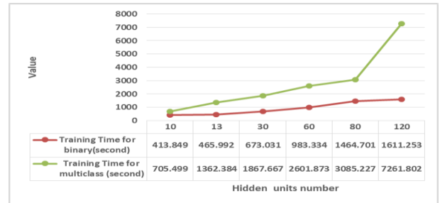
FIGURE 9. The training time on KDDTRAIN+ dataset in the binary and multiclass classification with different number of hidden units.
