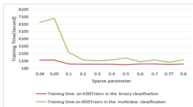
FIGURE 11. The training time on KDDTRAIN+ dataset in the binary and multiclass classification with different sparse parameter.
