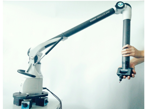
FIGURE 9. The articulated arm coordinate measuring machine used in experiments.
