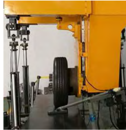
FIGURE 3. Experimental setup of the tire longitudinal properties.
