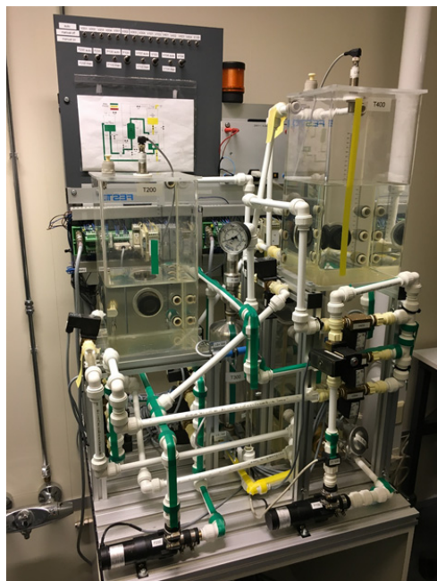
FIGURE 10. Heat production plant process (HPP) used as a testbed for the proposed method.
