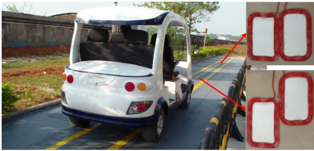
FIGURE 13. EV-DWPT system prototype.
