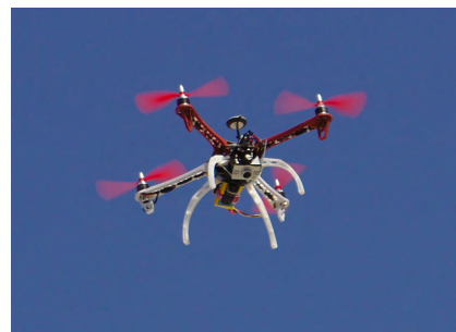
FIGURE 10. DJI F-450 drone equipped with a Nilox F60 camera, used for acquiring the MIVIA Drone dataset.
