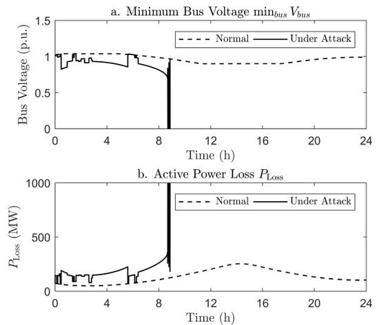
FIGURE 6. Single substation attack: (a) minimum bus voltage during attack and (b) active power loss.
