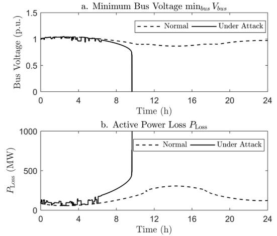
**FIGURE 7. Propagation attack: (a) minimum bus voltage during attack and (b) active power loss.**
