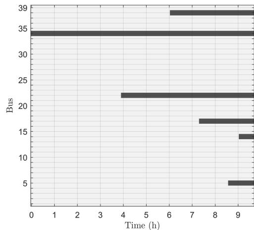
**FIGURE 8. Sequence diagram of virus propagation. Black bars indicate that the bus is infected. Buses #34, #22, #38, #17, #14, and #5 are successively infected.**
