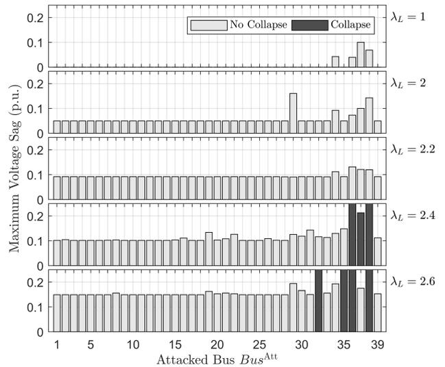
**FIGURE 10.** Single substation attacks in 195 scenarios. Maximum voltage sag is defined as  $\max_{t, bus} V_0 - V_{bus}(t)$ ,  $V_0 = [1, 1, \dots, 1]$ . The seven black bars indicate that in these seven scenarios, bus voltage drops below the operational limit of 0.8 p.u..
