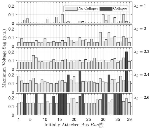
**FIGURE 9.** Propagation attacks in 195 scenarios. Maximum voltage sag is defined as  $\max_{t, bus} V_0 - V_{bus}(t)$ ,  $V_0 = [1, 1, \dots, 1]$ . The 19 black bars indicate that in these 19 scenarios, the bus voltage drops below the operational limit of 0.8 p.u..
