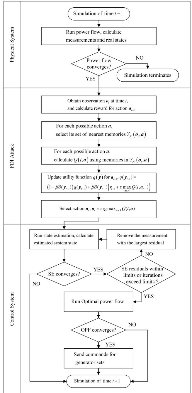
FIGURE 3. Flow diagram of FDI attack simulation.
