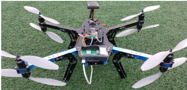
FIGURE 9. 3DR X8+ drone used for experiments.
