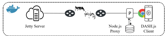
FIGURE 6. Experimental setup. MiniNet is used to host a virtual network within a Docker container. The DASH.js player is used in the Google chrome browser, starting and playing different video streaming sessions from the HTTP/2-enabled Jetty server.
