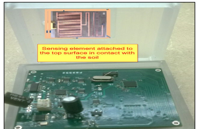
FIGURE 2. Sensor circuit inside the Package.
