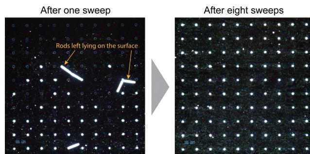
**FIGURE 7. Top-view optical microscope images of the same array after one sweep and after eight sweeps. Filled holes can be clearly distinguished from the unfilled ones.**
