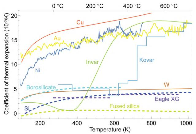
**FIGURE 9.** Instantaneous and semi-instantaneous CTEs of substrate materials (dashed lines) and conductor materials (solid lines) as a function of temperature.
