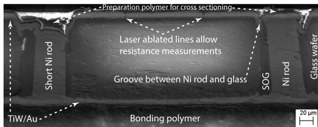
**FIGURE 4.** Cross section SEM showing a functional TGV pair. The lines cut in the metal layer on top of the wafer define the areas connecting adjacent TGVs in series for the purpose of resistance measurements (cf. Fig. 2f and 2j).
