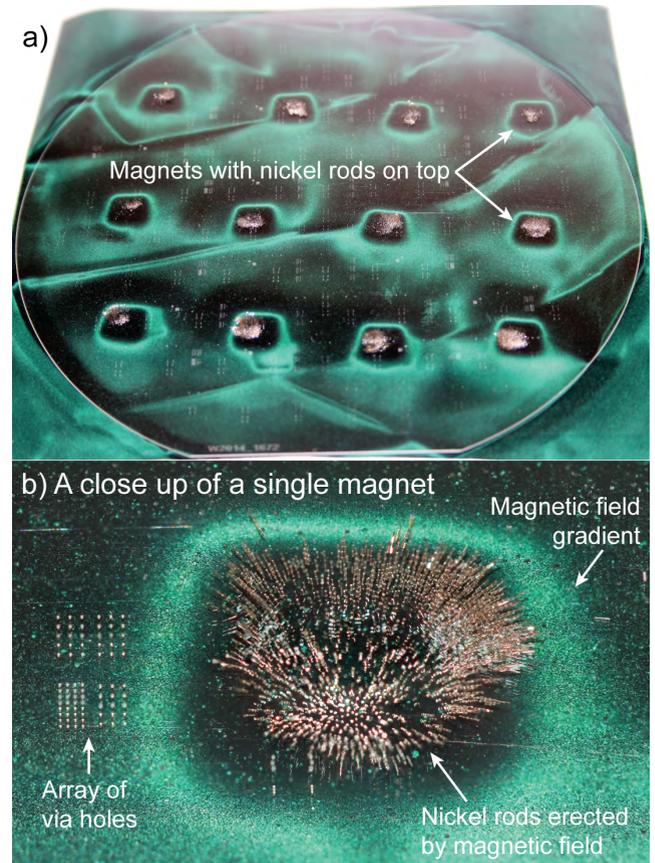
**FIGURE 1.** a) Photograph of a glass wafer with a magnetic sheet and twelve permanent magnets underneath. Between the magnets and the wafer is a flux-detector foil that visualizes the shape of the magnetic field. The foil contains nickel particles that show black in green gelatinous suspension. b) A close up of a single magnet with nickel rods on top and via holes ready to be assembled.
