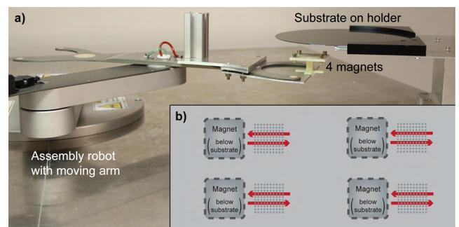
**FIGURE 3.** a) Setup for parallel assembly with a robot. b) Schematic top view of the movement of the magnets underneath hole arrays in a silicon substrate.
