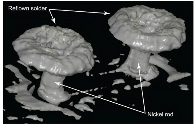
**FIGURE 5.** Computed tomography (CT) rendering of a TGV pair after successful reflow of the solder paste on top of the TGVs.
