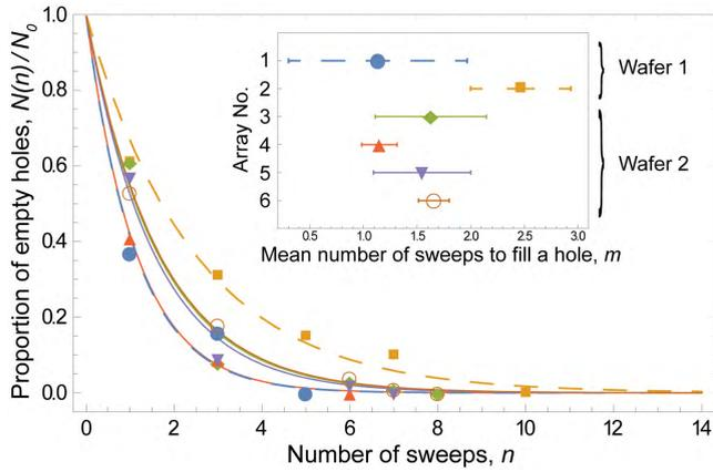
**FIGURE 8.** Measured ratio of empty holes in each array after a number of sweeps together with fits using the function in (1). Inset shows the mean number of sweeps needed to fill a single hole in each array together with 95% confidence limits.
