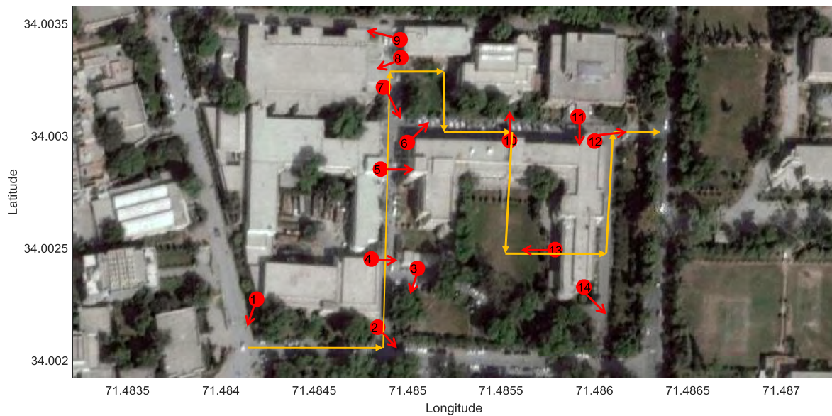
FIGURE 6. Campus Google map with CCTV cameras locations marked by red circles. The orange track is the path of the POI covered for testing.
