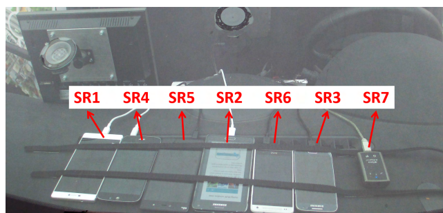
FIGURE 11. Placement of smartphones and Bluetooth receiver module behind the windshield.
