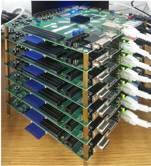
FIGURE 1. Xilinx Zynq-7000 FPGA boards.
