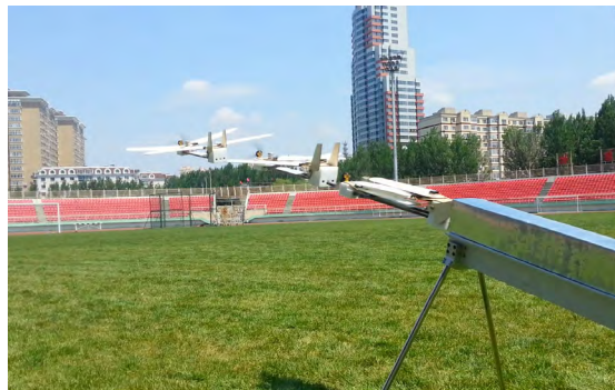
FIGURE 1. Catapult launch of the previous tandem-wing MAV prototype [26].
