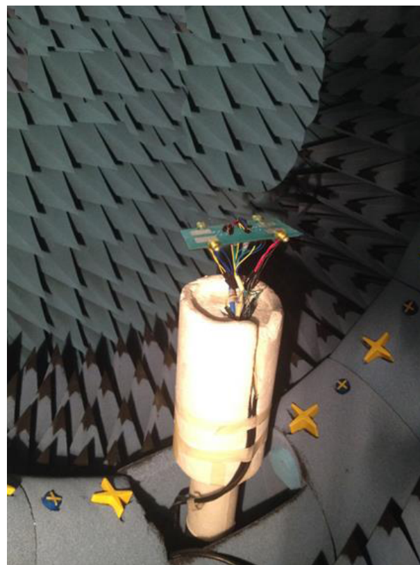
FIGURE 9. Setup for antenna radiation pattern measurement.
