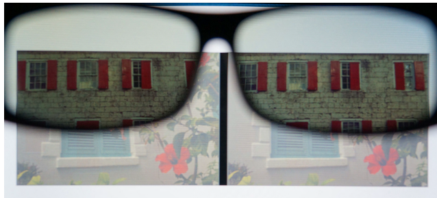
FIGURE 6. The views by the heuristic and iterative algorithms are presented side by side at the same time. The shared view and personal view can be seen with or without the glasses.
