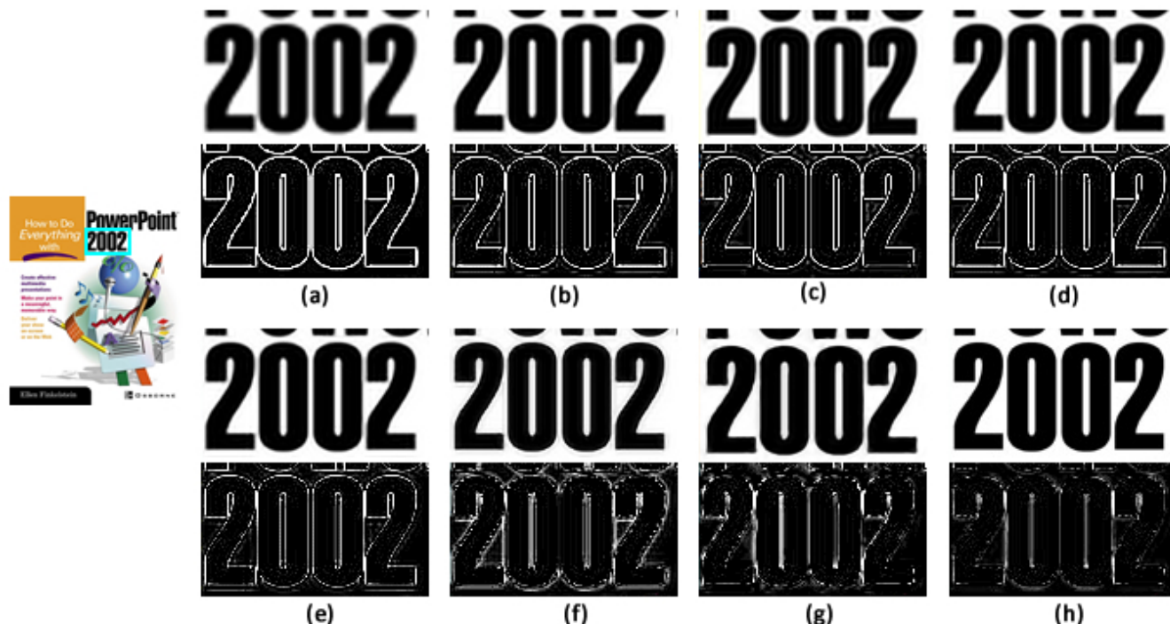
FIGURE 9. 2x SR results of ‘PPT’ image with different methods, (a) with bicubic, (b) with the LLE [26], (c) with the ASDS [32], (d) with the ANR [42], (e) with the A+ [43], (f) with the SRCNN [44], (g) with the VDSR [45], (h) with the GUN. The residual map between each result and the original HR image is illustrated.
