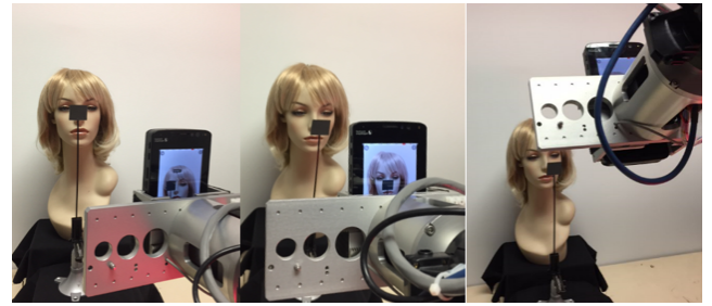
FIGURE 12. Robotic arm moves the device to each position for face occlusion testing.
