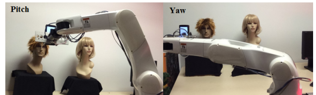
FIGURE 9. Robotic arm at pitch and yaw angles on mannequin No. 2.
