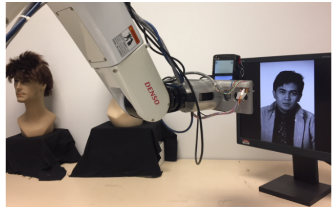
FIGURE 13. 2D face image testing on display monitor.
