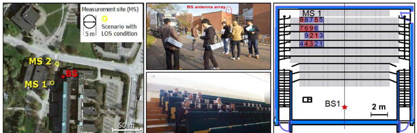
FIGURE 1. (Left) Aerial photo of the outdoor measurement area showing the location of the BS (on a roof top) and the user sites (yellow circles). Users are confined to the area within the yellow circles. (Middle-top) Users at site MS 1 move in random trajectories. (Middle-bottom) Nine users sitting in lecture theater E:A. User antennas are being held with a 45^\circ downtilt and move in random trajectories. (Right) Floor plan of lecture theater E:A.
