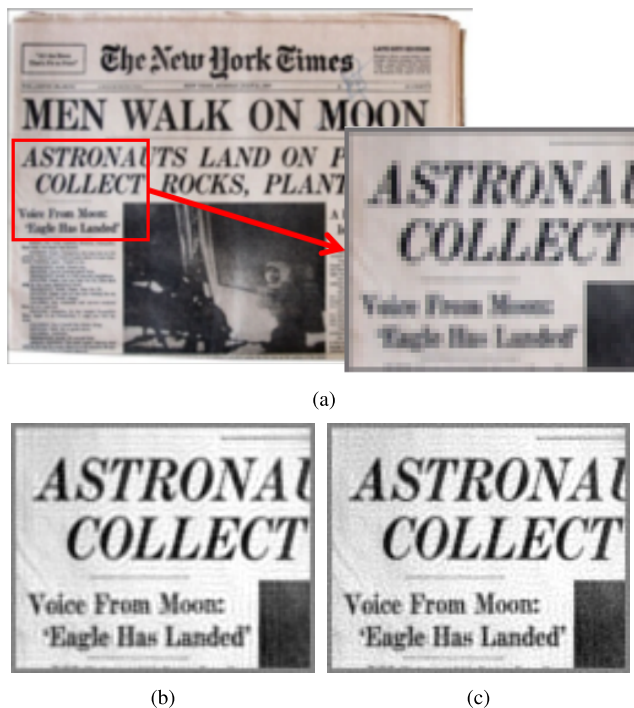
FIGURE 12. SR method applied for restoration of information in newspaper texts. Comparison of the enhancement of the edge elements of our proposal in relation to the SAR model. LR image adapted from [46]. (a) LR image. (b) SAR. (c) SARM.
