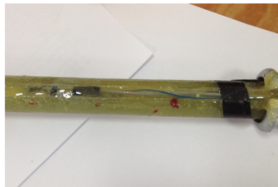
FIGURE 8. The temperature probe embedded in the core.
