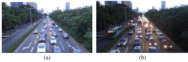
FIGURE 7. The normal and abnormal traffic screenshot in Scene 2. (a) Slight traffic congestion. (b) Heavy traffic congestion.
