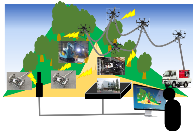
FIGURE 7. The framework of our cloud robotic cooperation system.
