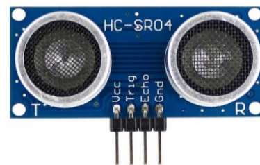
FIGURE 1. Ultrasonic Ranging Module HC - SR04.
