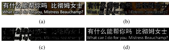
FIGURE 7. Result of FCM clustering. (a) Candidate text region. (b) Background layer. (c) Border layer. (d) Candidate text layer.
