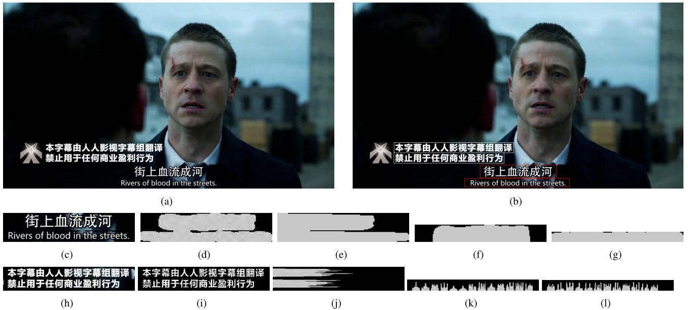
FIGURE 6. Candidate text line localization. (a) Original frame. (b) Localization result of the candidate text lines. (c) Candidate text region 1. (d) Corresponding contour 1. (e) Horizontal projection on contour 1. (f) Vertical projection on the first partitioned part. (g) Vertical projection on the second partitioned part. (h) Candidate text region 2. (i) Gray-scale image of candidate text layer extracted by the proposed FCM-based separation algorithm on candidate text region 2. (j) Horizontal projection on the gray-scale image. (k) Vertical projection on the first partitioned part. (l) Vertical projection on the second partitioned part.
