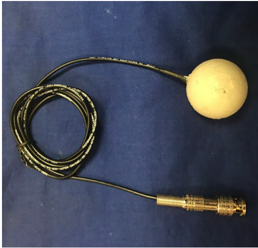
FIGURE 1. The fabricated spherical smart aggregate and its schematic.
