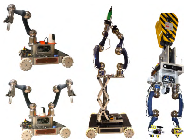
FIGURE 18. CERNbot v1.0 in single and dual arms configuration (left). CERNbot v2.0 with lifting stage in dual arms configuration (middle). CERNbot core (CRANEbot) in dual arms configuration (right).
