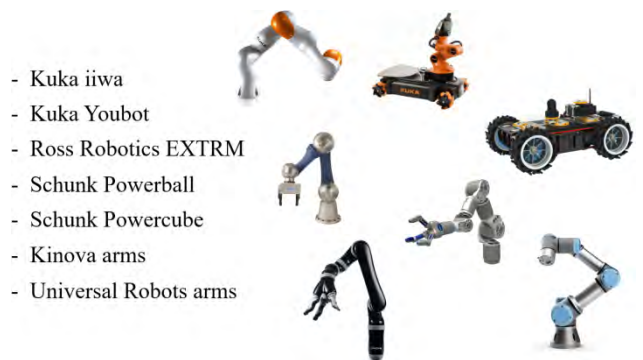
FIGURE 17. Robotic arms controlled by the CERNTAURO framework.
