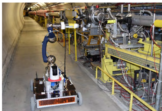
FIGURE 22. CERNbot doing autonomous radiation mapping of accelerator areas at CERN.
