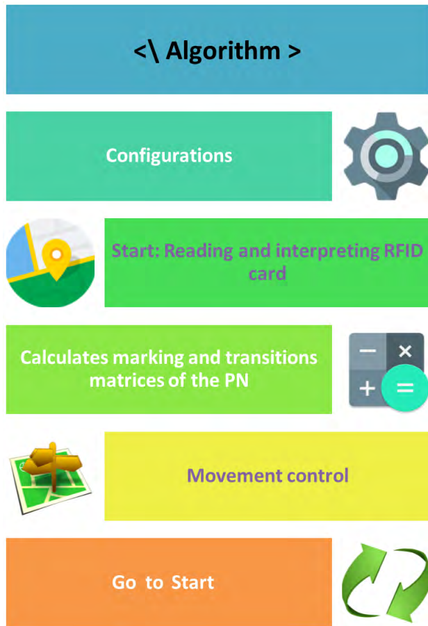
FIGURE 4. Logical sequence that controls the actions of the mobile robot.
