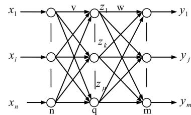
FIGURE 4. Three-layer BP neural network structure.
