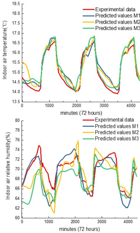
FIGURE 8. Comparison of experimental data and predicted values of IT and IH for 72 hours prediction.
