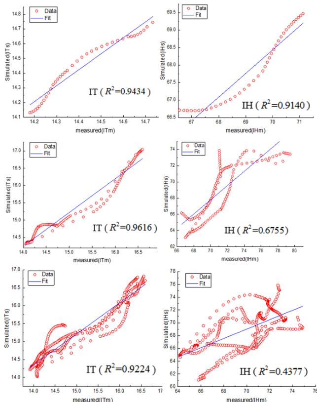
FIGURE 10. Regression lines between measured values and values predicted 6 h, 24 h, and 72 h ahead of M2.
