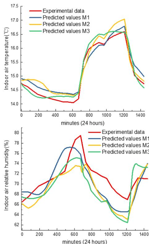
FIGURE 7. Comparison of experimental data and predicted values of IT and IH for 24 hours prediction.
