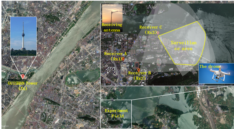
FIGURE 7. Scenario of drone detection experiment trial.
