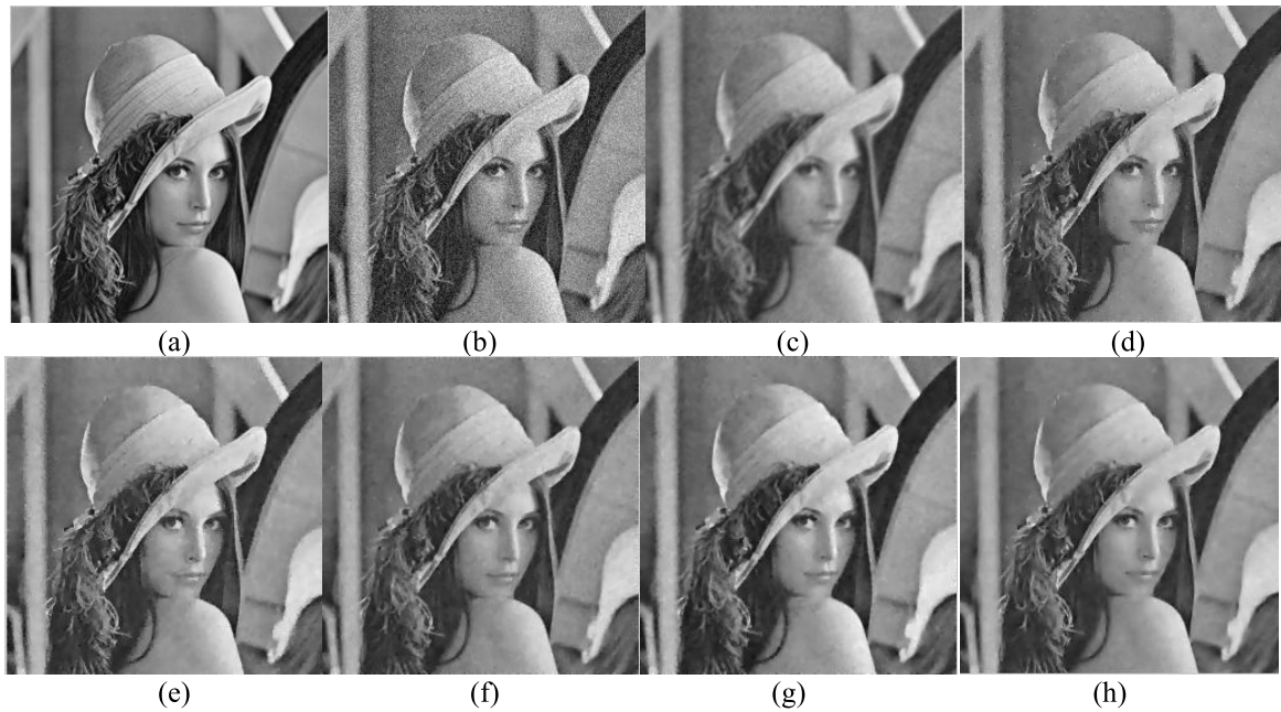
FIGURE 5. Comparison of denoising resultson Lena image. (a) noise free image; (b) noisy image with variance of 0.003; Denoising results by (c) ID model, (d) PM model ( k = 6 ), (e) VEPM model ( k = 4 ), (f) MPM model, (g) TSP model ( k = 5 ), as well as (h) DLHPDE model ( k = 2 ).
