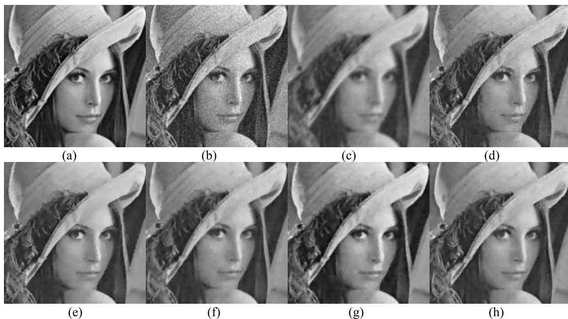
FIGURE 4. Comparison of denoising results for zoomed-in region of the Lena image. (a) noise free image; (b) noisy image with variance of 0.002; Denoising results by (c) ID model, (d) PM model ( k = 6 ), (e) VEPM model ( k = 4 ), (f) MPM model, (g) TSP model ( k = 5 ), as well as (h) DLHPDE model ( k = 2 ).
