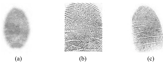
FIGURE 5. Three impressions of the same fingerprint from the MOLF database. (a) Lumidigm Venus IP65 Shell optical sensor. (b) Secugen Hamster-IV optical sensor. (c) CrossMatch L-Scan Patrol optical sensor
