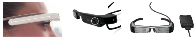
FIGURE 6. Trackpad on spectacle frame (Left), Button (Middle), external controller wired with Espon smart glasses (Right).
